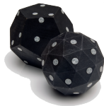
Figure 1.3: Examples of two general-purpose tracking targets. Notice how multiple markers are clearly visible from a single viewing angle.
